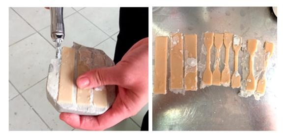
Figure 2. Divesting resin samples.
